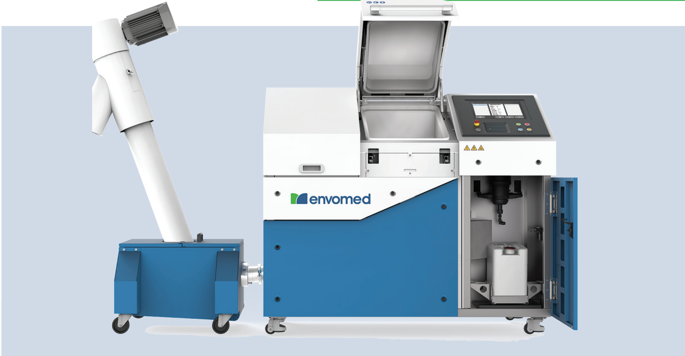
Envomed 80 - demonstrating the automatic use of Biocetic in the machine for sterilization of Medical Waste.
